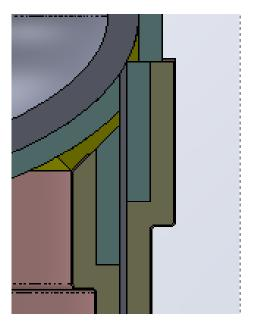
The above drawing illustrates the termination of the Calcium silicate. This is a typical view showing the ContraFlame® material on top of the calcium silicate for J30 10mm thick C50 and for H120 50mm thick. The above image shows 50mm thick C50.
