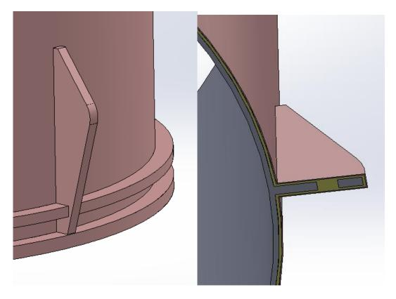
The above picture shows a typical termination of the ContraFlame® JF30 system to tailing lugs.
