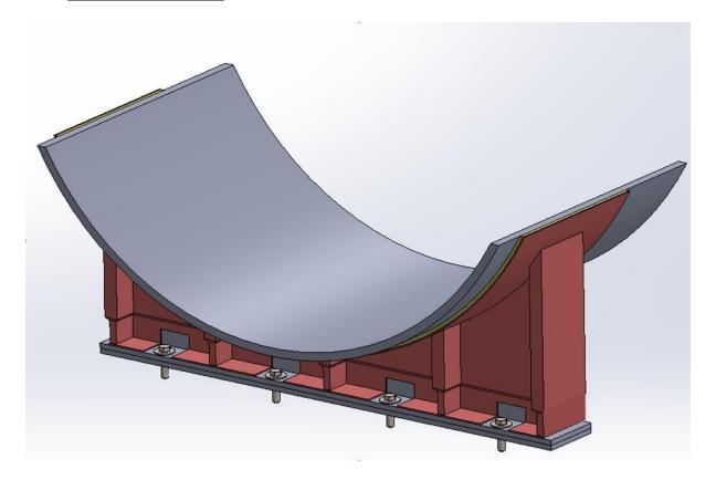
The above picture shows a typical termination of the ContraFlame® JF30 system to saddles on horizontal vessels.
