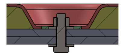
The above picture shows a typical termination of the ContraFlame® JF30 system to vessel anchor bolts.
