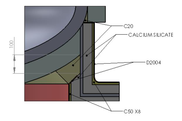
The above picture shows a typical termination of the ContraFlame® JF30 system to the inside and outside of the skirts on a hot vessel.
