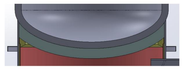
ContraFlame C20 material will be used to fill the void between the termination of the ContraFlame® JF30 system and Insulation.
