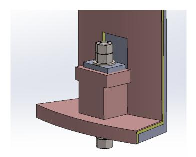
The above picture shows a typical termination of the ContraFlame® JF30 system to vessel anchor chairs.
