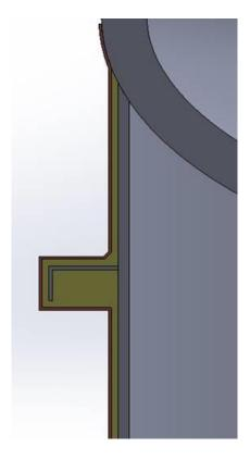
The above picture shows a typical termination of the ContraFlame® JF30 system to steel supports located on the skirts.
